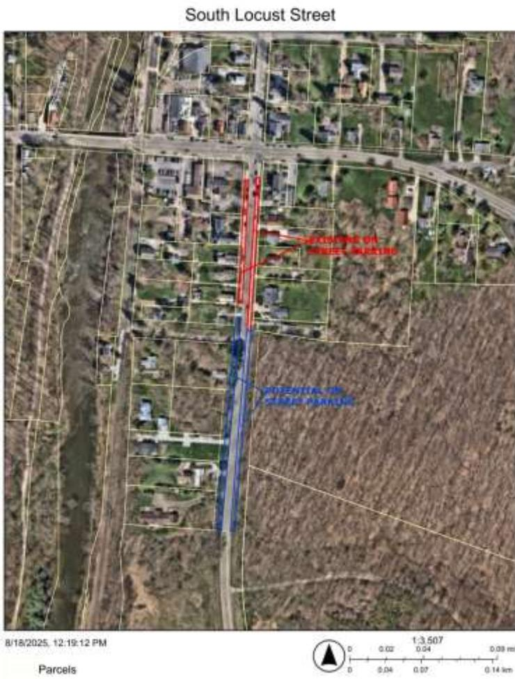
Valley National Park property. A total gain of 41 spaces could be achieved. The street pavement would have to be widened and a sidewalk would need to be installed on each side of the street for safety.
